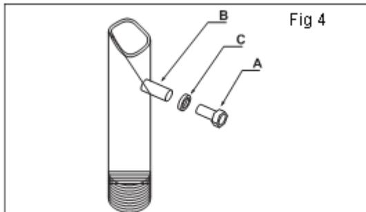
Gas supply pressure must be measured at the pressure point (Fig. 4)-(Ref. B) after removing the sealing screw (Ref. A). Use a flexible pipe, connect a gauge e.g. a liquid gauge that is accurate to 0.1 mbar) to the pressure point (and measure the intake pressure whilst the appliance is operating. If the pressure reading does not fall within the upper and lower limits indicated on the table, the appliance cannot be installed.
